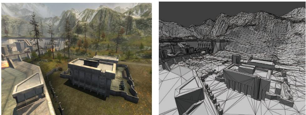
Figure 2. Boundary representation of C-Space for an outdoor environment with buildings
